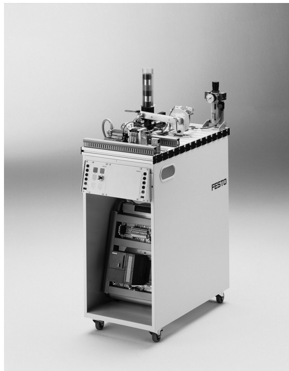
Distribution station with trolley, control console and PLC board
